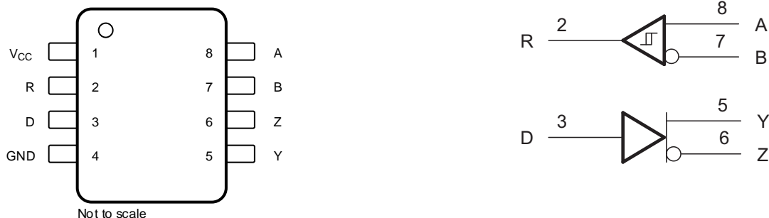
Pin Functions — SOIC-8 and MSOP-8
