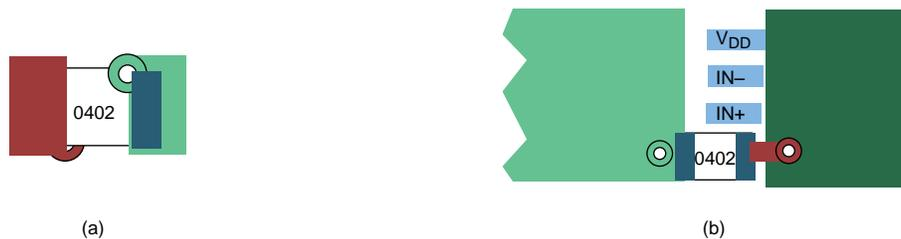
Figure 29. Typical Decoupling Capacitor Layouts
