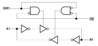
Figure 4. Logic Diagram (Positive Logic)
