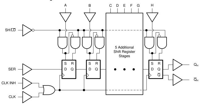
Figure 8-1. Logic Diagram (Positive Logic)
