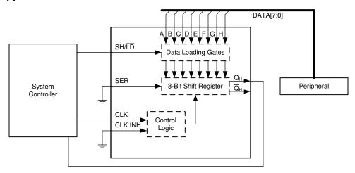
Figure 9-1. Input Expansion with Shift Registers
