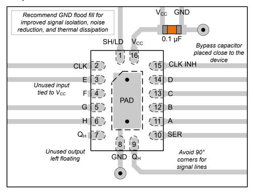
Figure 11-1. Layout Example for the SN74LV165A-Q1 in the WBQB Package
