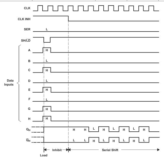
Figure 6-1. Typical Shift, Load, and Inhibit Sequences
