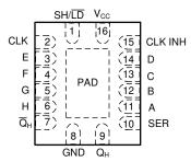
Figure 5-1. SN74LV165A: WBQB Package, 16-Pin WQFN (Top View)
