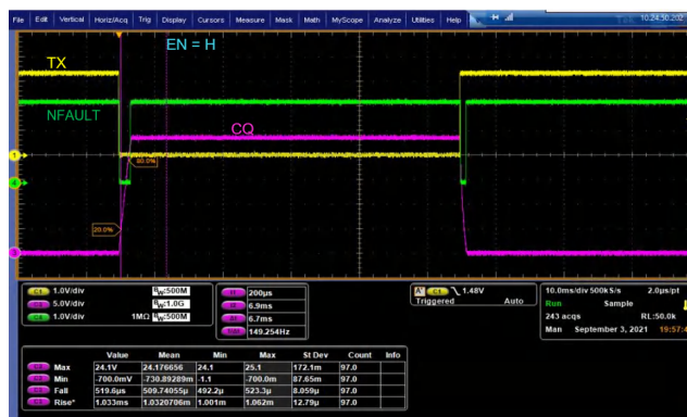
图 9-6. CQ Driving Inductive Load, Low Side Mode (NPN mode)
