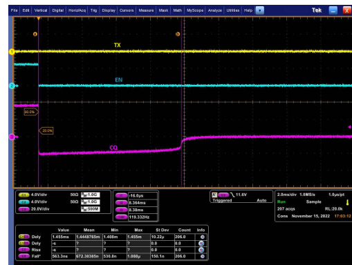
图 9-5. CQ in Current Fault Auto Recovery, High Side Mode
