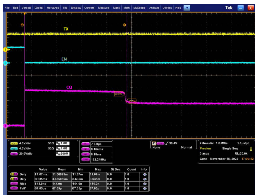
图 9-4. CQ in Current Fault Auto Recovery, Low Side Mode
