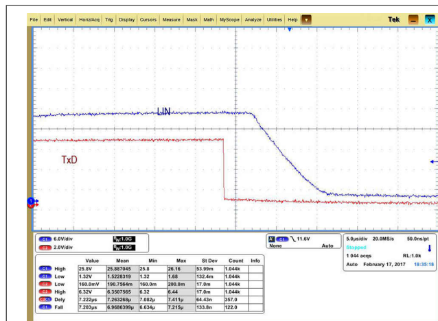
图 10-2. Recessive to Dominant Propagation
