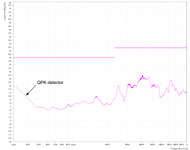
图 9-9. CISPR 32 Class B Radiated Emissions: Vertical Polarization
