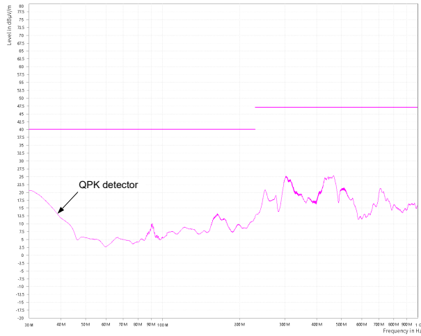
图 9-8. CISPR 32 Class B Radiated Emissions: Horizontal Polarization
