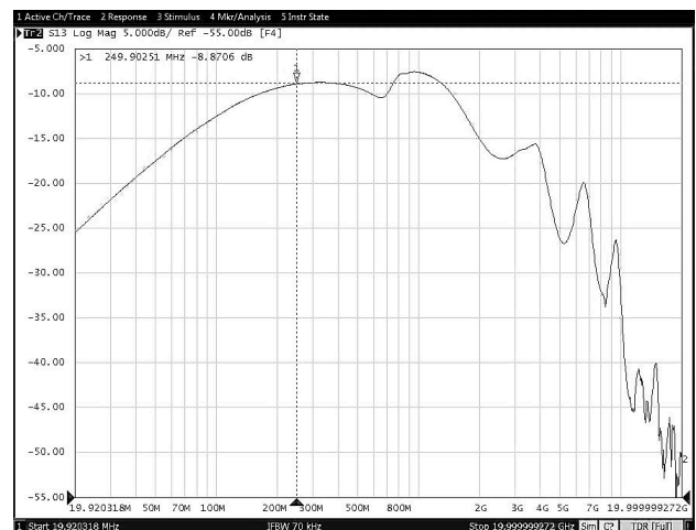
图 8-30. Off-State Data-Switch Isolation vs Frequency (TPS25830A-Q1)
