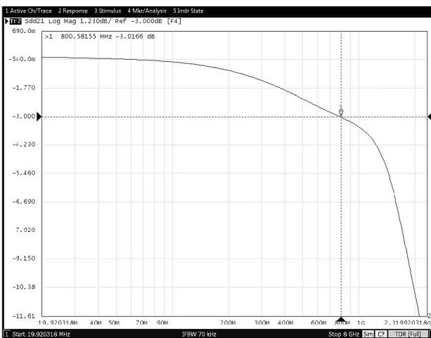
图 8-29. Data Transmission Characteristics vs Frequency (TPS25830A-Q1)
