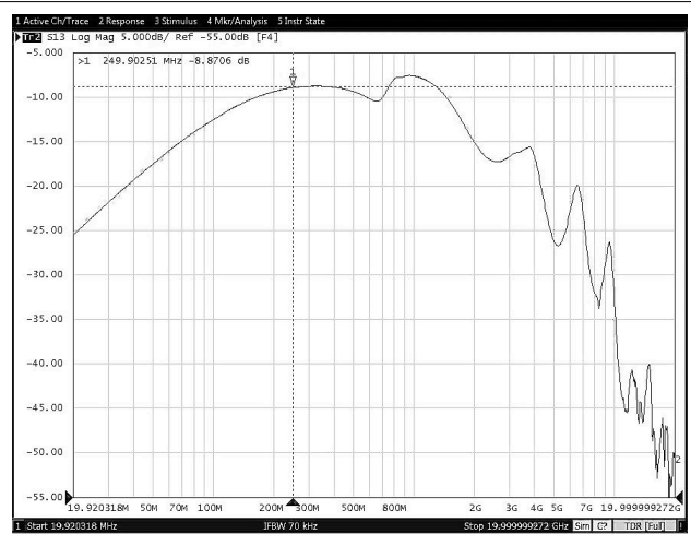
图 8-32. Off-State Data-Switch Isolation vs Frequency (TPS25830-Q1)
