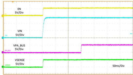
VIN = 0 V 至 13.5 V  $PA\_CC1 = R_d$   $I_{PA\_BUS} = 3A$
