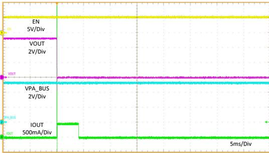
PA\_CC1 =  $R_d$     OUT = GND    PA/B\_BUS 空载
