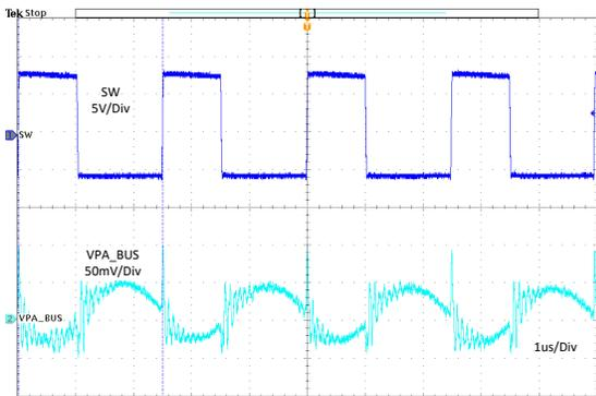
VSET = GND  $I_{PA\_BUS} = 3A$   $I_{PB\_BUS} = 3A$   $f_{SW} = 400kHz$
