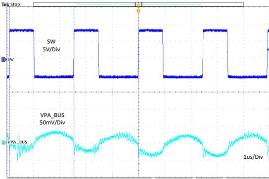
VSET = GND  $I_{PA\_BUS} = 0A$   $I_{PB\_BUS} = 0A$   $f_{SW} = 400kHz$
