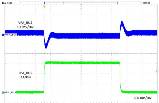
VSET =  $I_{PA\_BUS} = 0A$  至  $3A$   $I_{PB\_BUS} = 3A$   $f_{SW} = 400kHz$
