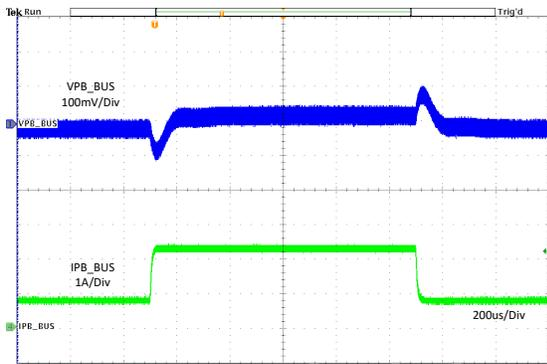
VSET =  $I_{PB\_BUS} = 0.75A$  至 GND  $I_{PA\_BUS} = 0A$   $f_{SW} =$
