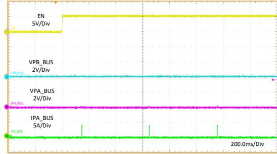
EN 至高电平 PA\_BUS = GND PB\_BUS = GND
