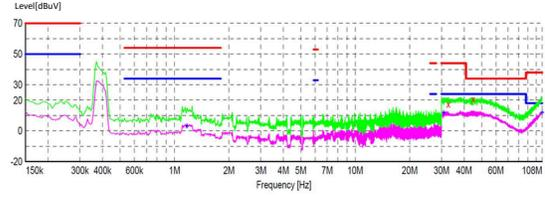
PA\_BUS = 3A,  $f_{SW} = 400kHz$   $L = 3.3\mu H$
