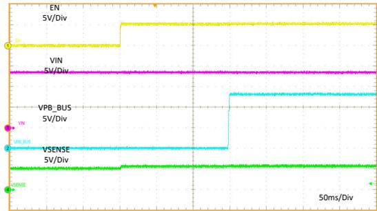
EN = 0V 至 5V  $PB\_CC1 = R_d$   $I_{PB\_BUS} = 3A$
