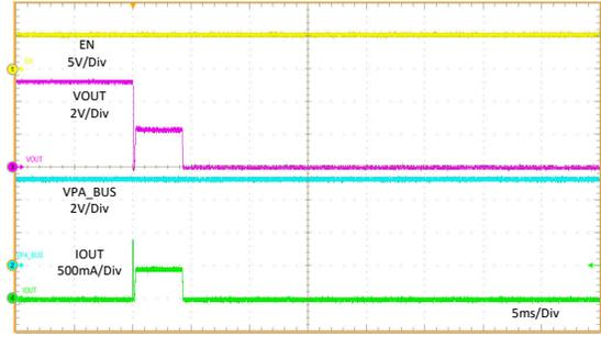
PA\_CC1 =  $R_d$     OUT = 5.1  $\Omega$     PA/B\_BUS 空载
