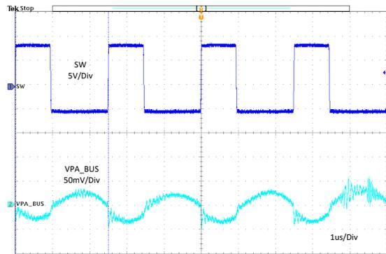
VSET =  $I_{PA\_BUS} = 0.1A$   $I_{PB\_BUS} = 0A$   $f_{SW} = 400kHz$
