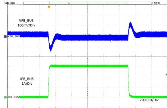
VSET =  $I_{PB\_BUS} = 0A$  至  $3A$   $I_{PA\_BUS} = 3A$   $f_{SW} = 400kHz$
