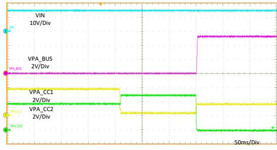
$PA\_CC1 =$  开路至  $R_d$   $PA\_CC2 =$  开路  $I_{PA\_BUS} = 3A$
