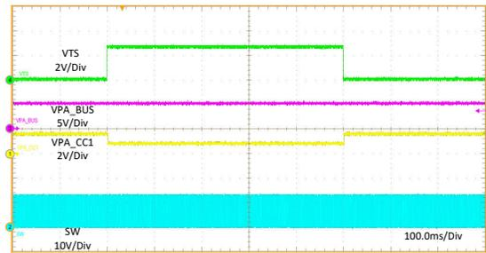
$V_{TS}$  = 0V 至 2.6V    PA\_CC1 =  $R_d$     PA\_CC2 = 开路
