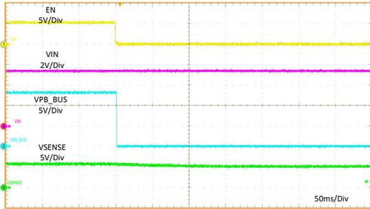
EN = 5V 至 0V  $PB\_CC1 = R_d$   $I_{PB\_BUS} = 3A$
