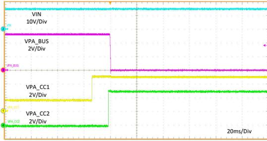
PA\_CC1 =  $R_d$  至开 PA\_CC2 = 开路  $I_{PA\_BUS} = 3A$
