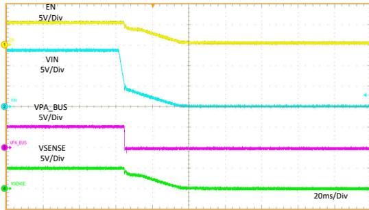
VIN = 13.5 V 至 0 V  $PA\_CC1 = R_d$   $I_{PA\_BUS} = 3A$
