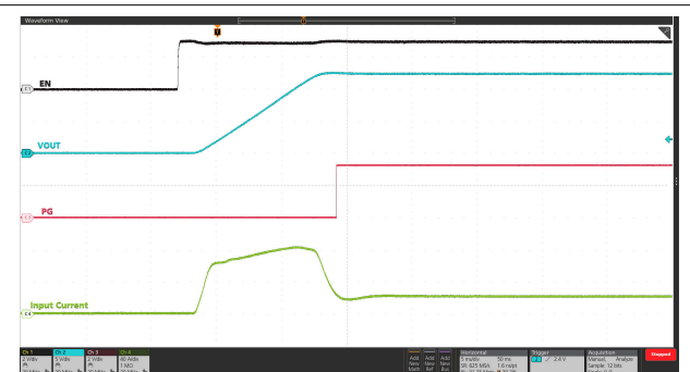
Figure 9-6. Start-up with EN/UVLO: V_{IN} = 12 V, EN/UVLO Stepped Up From 0 V to 3 V, C_{LOAD} = 50 mF, R_{LOAD(Start-up)} = 0.48 \Omega , C_{DVDT} = 33 nF, V_{IREF} = 1 V, R_{ILIM(TPS25990)} = 422 \Omega , and R_{ILIM(TPS25985)} = 316 \Omega
