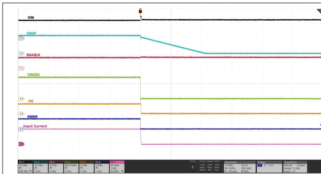
IN supply held steady at 12 V, EN pin held high, PMBus OPERATION OFF Command. C_{OUT} = 18\text{ mF} , C_{dVdt} = 33\text{ nF} Figure 7-37. Power Down Using PMBus Command
