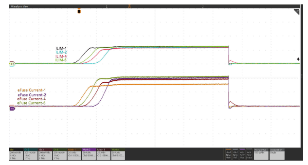
Figure 9-8. Power Up into Short (Current distribution among six devices in parallel): V_{IN} = 12 V, EN/UVLO Stepped Up From 0 V to 3 V, V_{IREF} = 1 V, R_{ILIM(TPS25990)} = 422 \Omega , R_{ILIM(TPS25985)} = 316 \Omega , and OUT Shorted to GND
