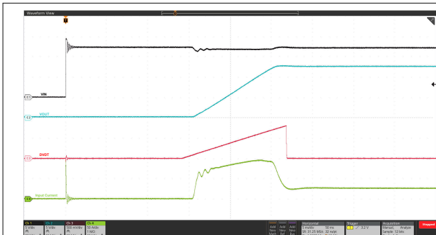
Figure 9-5. Input Hot Plug: V_{IN} Stepped Up from 0 V to 12 V, C_{LOAD} = 50 mF, R_{LOAD(Start-up)} = 0.48 \Omega , C_{DVDT} = 33 nF, V_{IREF} = 1 V, R_{ILIM(TPS25990)} = 422 \Omega , and R_{ILIM(TPS25985)} = 316 \Omega
