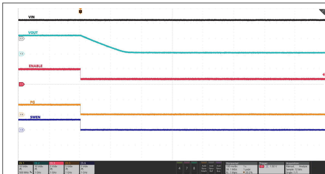
Figure 7-43. Power Down Using EN With Output Discharge
