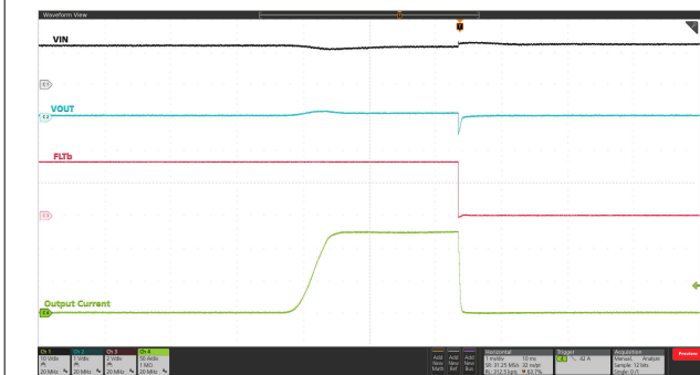
Figure 9-7. Power Up into Short: V_{IN} = 12 V, EN/UVLO Stepped Up From 0 V to 3 V, V_{IREF} = 1 V, R_{ILIM(TPS25990)} = 422 \Omega , R_{ILIM(TPS25985)} = 316 \Omega , and OUT Shorted to GND
