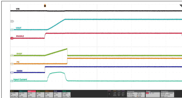
IN supply held steady at 12 V, EN toggled from low to high. C_{OUT} = 18 \text{ mF} , C_{dVdt} = 33 \text{ nF} , Default PG delay setting ( DEVICE_CONFIG[15] = 0b )
