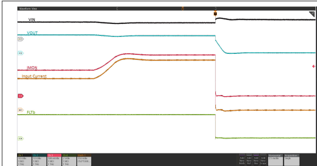
Figure 9-11. Circuit-Breaker Response: V_{IN} = 12\text{ V} , t_{OC\_TIMER} = 10\text{ ms} , C_{LOAD} = 50\text{ mF} , R_{IMON} = 150\ \Omega , V_{IREF} = 1\text{ V} , and Load Current Stepped from 333 A to 530 A for more than 10 ms
