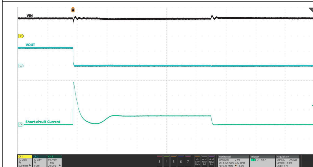
Figure 7-57. Short-Circuit Protection During Steady-state
