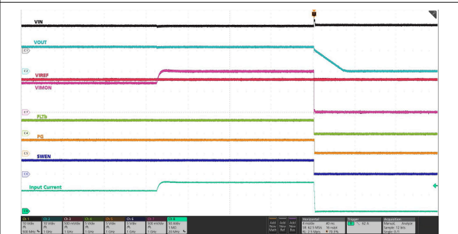
Device in steady-state, Load current ramped up from 50 A to 70 A for > 15 ms. OCP threshold set to 55 A, Overcurrent blanking delay set to 15 ms ( OC_TIMER = 0x89 )
