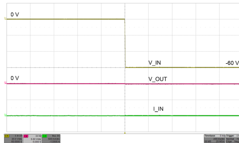
Figure 36. Reverse Input Supply Protection at -60 V
