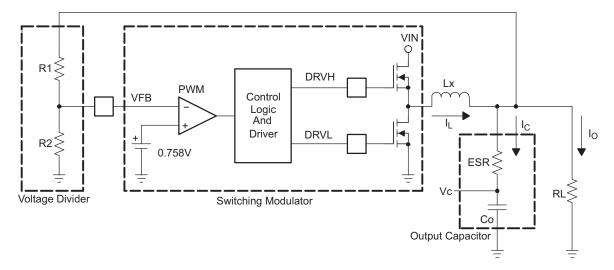
Figure 19. Simplifying the Modulator
