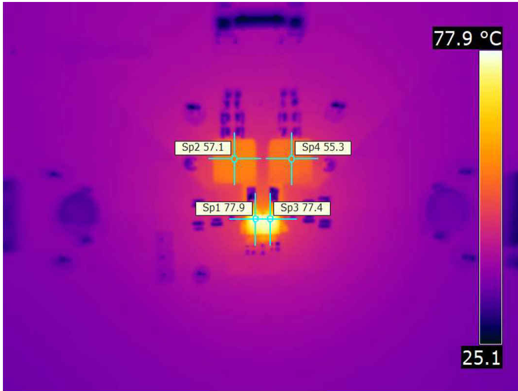
图 10-4. Thermal Image at 25°C Ambient - Dual Output Operation, f_{sw} = 1 \text{ MHz} , V_{IN} = 12 \text{ V} , V_{OUT1} = 1 \text{ V} , I_{OUT1} = 6 \text{ A} , L_1 = 560 \text{ nH} (3.3 m \Omega Max), V_{OUT2} = 3.3 \text{ V} , I_{OUT2} = 6 \text{ A} , L_2 = 1.2 \text{ } \mu\text{H} (7.5 m \Omega Max)
