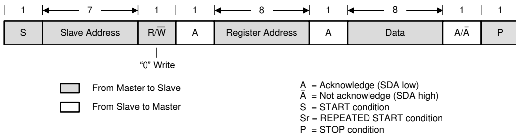
图 8-6. “Write” Data Transfer Format in Standard-, Fast, and Fast-Plus Modes
