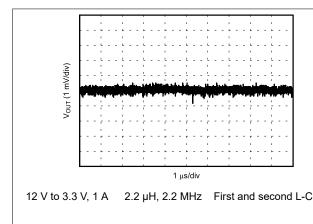
Figure 6-13.  $V_{OUT}$  Ripple After the Second L-C Filter
