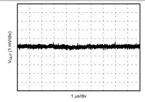
12 V to 1.2 V, 1 A 2.2 µH, 1 MHz First and second L-C With Random Spread Spectrum Enabled
