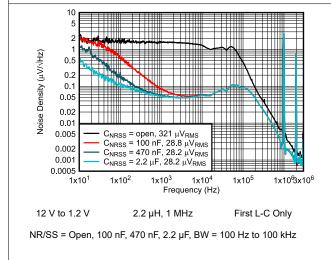
Figure 6-29. Output Noise Density vs Frequency
