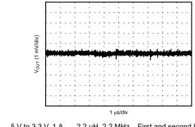
5 V to 3.3 V, 1 A 2.2 µH, 2.2 MHz First and second L-C
