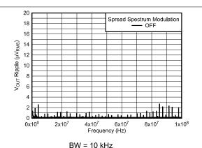
5 V to 3.3 V, 1 A 2.2 µH, 2.2 MHz First and second L-C
