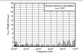
Figure 6-16. V<sub>OUT</sub> Ripple FFT After the First L-C Filter
