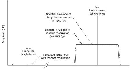
Figure 7-2. Spread Spectrum Modulation
