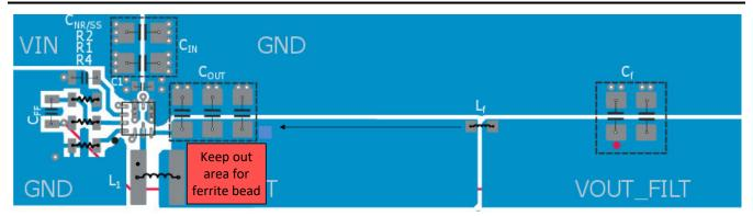
Figure 10-2. Recommended Layout for Design with Second L-C Filter
