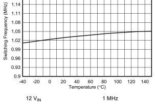
Figure 6-54. Oscillator Frequency vs Temperature
