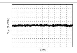
12 V to 1.2 V, 1 A 2.2 µH, 1 MHz First and second L-C
