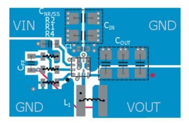
Figure 10-1. Recommended Layout for Single L-C Filter
