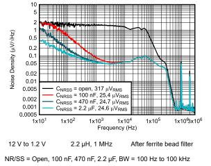
Figure 6-30. Output Noise Density vs Frequency
