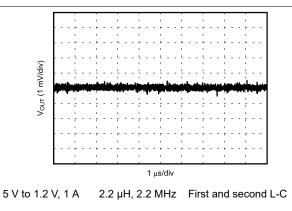
Figure 6-17.  $V_{OUT}$  Ripple after the Second L-C Filter
