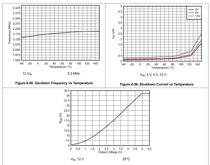
Figure 6-57. Output Discharge Resistance vs Output Voltage
