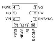
Figure 5-1. 10-Pin QFN RPU Package (Top View)
