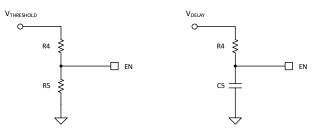
图 9-2. Circuit Example for How to Use the Precise Device Enable Feature
