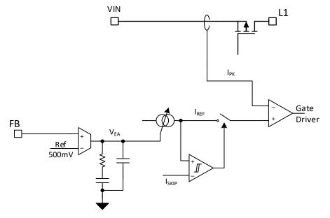
图 9-1. Control Loop Architecture Scheme
