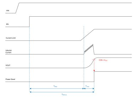
图 9-4. Device Start-up Scheme
