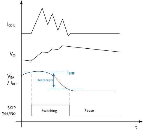
图 9-10. Power Safe Mode Operation Curves
