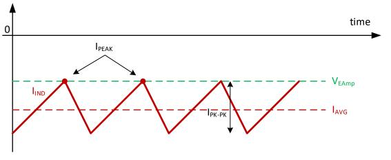
图 9-6. Peak-Current Operation, Reverse Current
