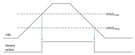
图 9-3. Rising and Falling Undervoltage Lockout Behavior
