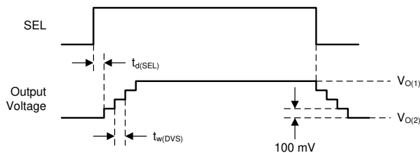
Figure 7-10. Dynamic Voltage Scaling with High Load
