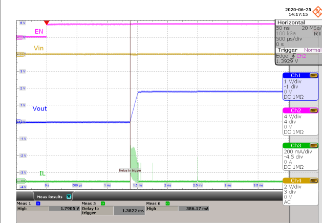
Figure 8-27. Load Transient, 300 mA Step
