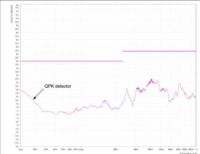
图 9-11. CISPR 32 Class B Radiated Emissions: Vertical Polarization
