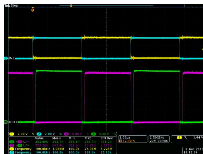
Figure 41. Bench Test Waveform for INA/B and OUTA/B
