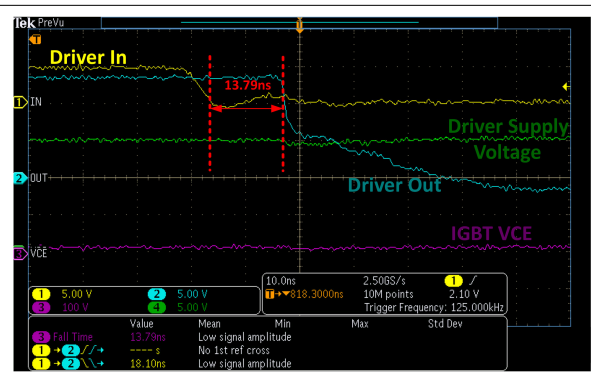
Figure 8-3. UCC27624 Used to Drive IGBT in the Boost Converter
