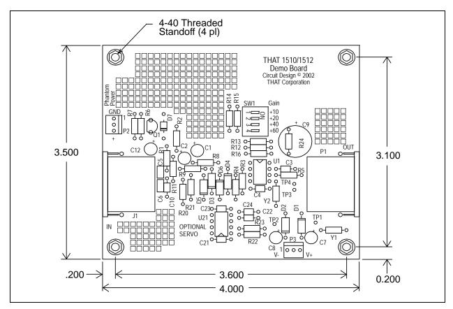
Figure 1. THAT 1510/12 Demonstration System Layout
