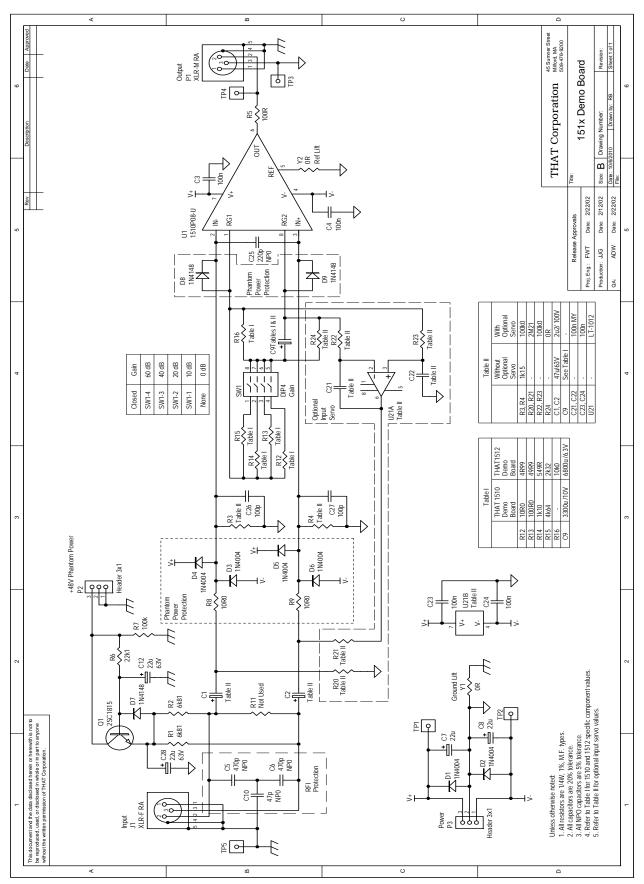
Figure 2. THAT 1510/1512 Demonstration System Schematic
