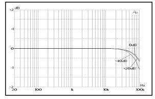
Figure 3. 2180-series Frequency Response vs. Gain
