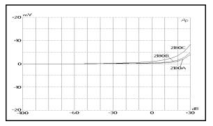
Figure 9. Representative DC Offset vs. Gain
