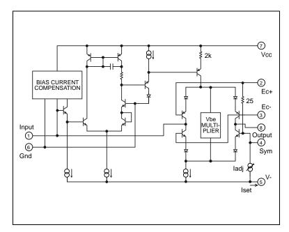
Figure 1. 2180-series equivalent circuit diagram
