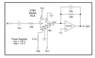
Figure 14. Positive control port using Pin 2 (E<sub>C+</sub>)
