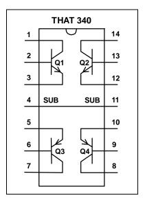
Figure 1. 300 Pinout
