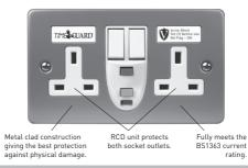
The RCD socket comes in two forms, a latching (passive) version with the penultimate letter set to 'P' in the type number and a non-latching (active) version which has the penultimate letter set to 'A'.
