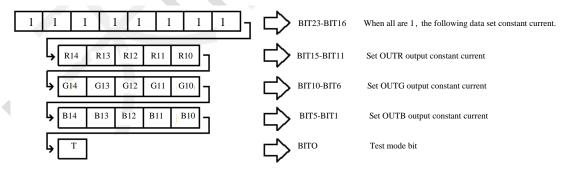
RI [bit15~bit11]:Set R channel constant-current value, Ir=10+RI[4:0]mA, namely minimum 10+0=10mA, maxium 10+31=41mA
