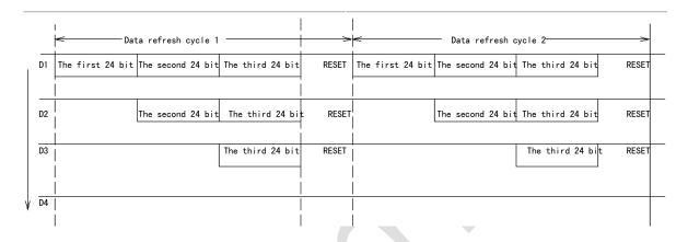
Chip cascade, data transmission and retransmission procedure: Data (D1) is sent from controller. When chip 1 finishes receiving the first 24bit, chip 1 does not retransmit data (D2) still and controller continues to send data, chip 1 receives the second 24bit. As the first 24 bit is existed in chip1, chip 1 retransmits the second 24bit out through DO. Chip 2 receives the data (D2) retransmitted from Chip1.At this time, chip 2 still does not retransmit data
