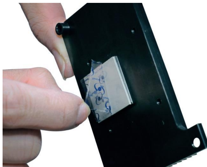
Figure 3: Remove plastic foil from the TIM
