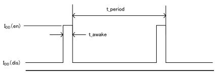
The Hall IC is operated intermittently to reduce supply current.
