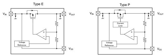
\* Diodes inside the circuits are ESD protection diodes and parasitic diodes.
