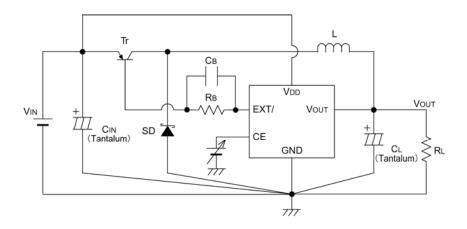
Circuit 6. XC6365B, XC6366B (when used with a PNP transistor)
