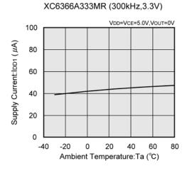
(8) Supply Current 2 vs. Ambient Temperature
