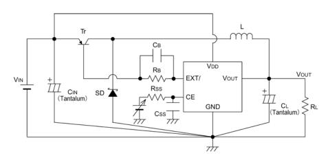
Circuit 8. XC6365D, XC6366D (when used with a PNP transistor)
