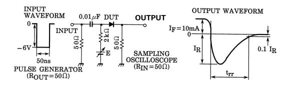
Fig.1 Reverse recovery time (t<sub>rr</sub>) test circuit
