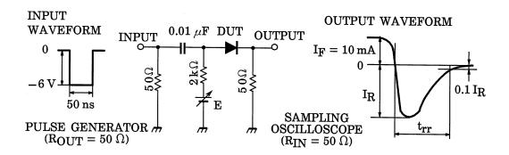
Fig.1 Reverse Recovery Time (t<sub>rr</sub>) Test Circuit
