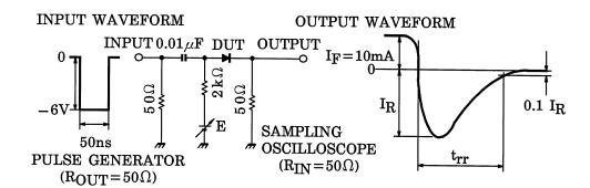
Fig.1 Reverse Recovery Time (t<sub>rr</sub>) Test Circuit
