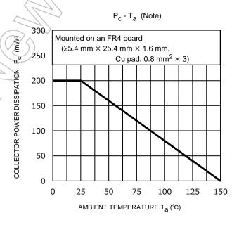
Note: The above characteristics curves are reference only with a junction temperature T $_{\rm j}$  of 150  $^{\circ}{\rm C}$ .
