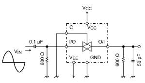
Figure 4 Feedthrough Attenuation
