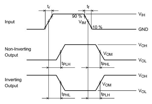
Fig. 12.8.1 t<sub>PLH</sub>, t<sub>PHL</sub>
