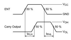
Figure 6 Cascade Mode (fix maximum count)
