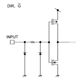
13. Bus Terminal Equivalent Circuit
