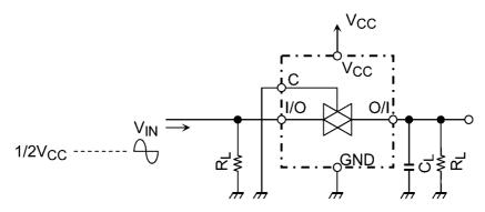
Figure 4 Feedthrough
