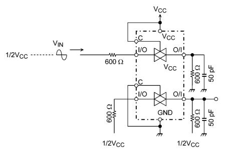
Figure 6 Cross Talk (between any two switches)
