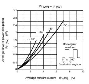
Device mounted on a ceramic board: board size: 50 mm × 50 mm Soldering land: 2 mm × 2 mm
