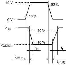
Fig. 5.3.1 Switching Time Test Circuit
