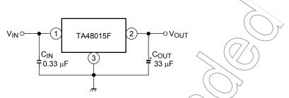
Be sure to connect a capacitor near the input terminal and output terminal between both terminals and GND. The capacitances should be determined experimentally. In particular, adequate investigation should be made so that there is no problem even in high or low temperatures.
