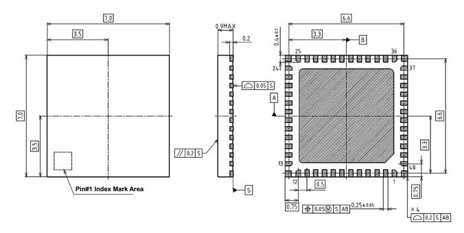
Backside heatsink: 5.4 mm × 5.4 mm
