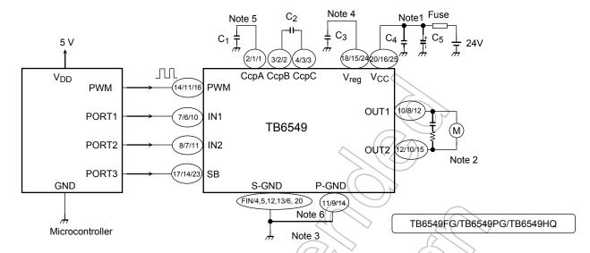
TB6549FG: Pins 1, 5, 6, 9, 13, 15, 16, and 19 are not connected.
