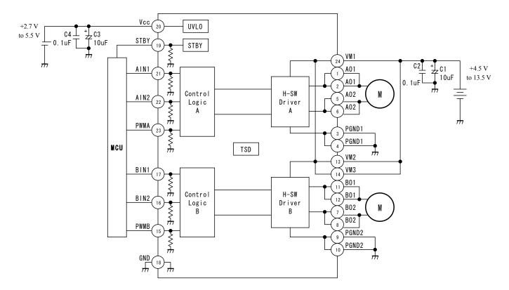
Note: Condensers for noise absorption (C1, C2, C3, and C4) should be connected as close as possible to the IC.
