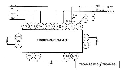
Note 1: Connect the V<sub>S2A</sub> terminal to the lower supply voltage (5 V).
