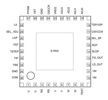
Note 1: Design the pattern in consideration of the heat design because the back side (E-PAD (3.4 mm × 3.4 mm)) and the four corners of the PAD have the role of heat radiation. (The back side (E-PAD) and the four corners of the PAD should be connected to GND because they are connected to the back of the chip electrically.)
