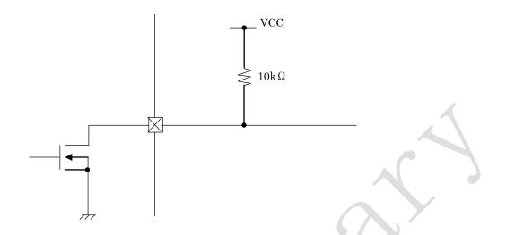
The LO is an open-drain output pin. LO pin needs to be pulled up to 3.3V/5.0V level for proper function. During regular operation, the LO pin level will stay High(VCC level). When error detection (TSD, ISD) is applied, the LO pin will show Low (GND) level.
