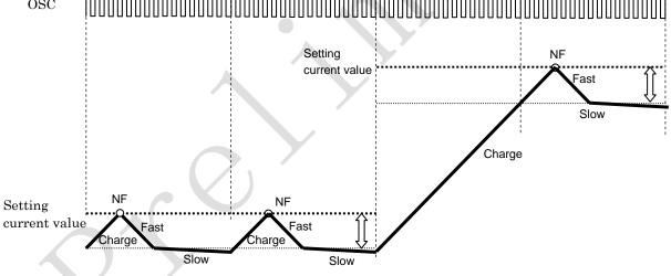
When the Charge period is longer than fchop cycle, the Charge period will be extended until the motor current reaches the NF threshold. Once the current reaches the next current step, then the sequence will go on to decay mode.
