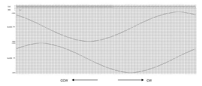
MO output shown in the timing chart is when the MO pin is pulled up.
