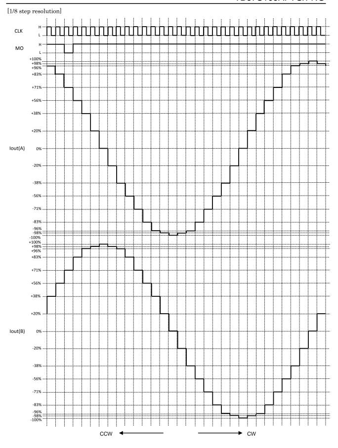
$\ensuremath{\mathrm{MO}}$  output shown in the timing chart is when the  $\ensuremath{\mathrm{MO}}$  pin is pulled up.
